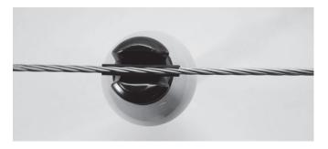
**2.** Install Distribution Tie onto insulator so both legs are parallel to the conductor.
