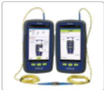
AFL's ROGUE OLTS Certifier measures insertion loss, return loss and length bi-directionally to industry standards on both multimode and single-mode networks. ROGUE OLTS Certifier is offered as a matched pair of units, with each unit featuring four test ports. Two of the ports combine a light source and power meter to enable bi-directional testing on single or dual fibers. The other two ports are a dedicated power meter and a visual fault identifier (VFI) to help troubleshoot networks.
