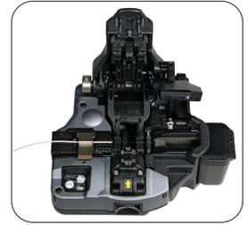
5: Set the fiber on the cleaver at the 10.5 mm recommended cleave length (minimum 10 mm). Cleave the fiber.
