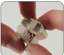
**7:** Place the connector into the assembly tool. Squeeze top and bottom of the wedge to ensure that it is engaged. (If using the optional VFI Method, see step 5b on page 2.)
