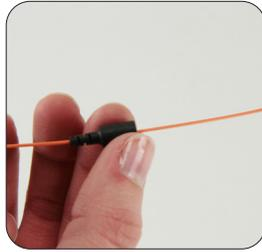
2: Place the 900 μm boot on the cable.
