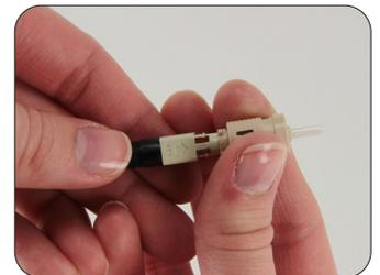
Before applying the connector housing to the connector body, ensure optical connection by the VFI or other suitable method. After the ST housing is applied, you will not be able to release/re-engage the wedge clip if resetting the fiber is required.
