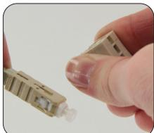
**9:** Release the wedge clip by squeezing both sides. Remove the wedge clip.
