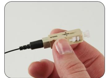
4: Slide the boot onto the connector body. Bring the clear protective tubing over the end of the 250  $\mu$ m protective tubing. Termination is complete.
