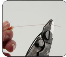
**4:** Strip off 35 mm of 900 µm and 250 µm coating. (Refer to template image on bottom of page 3 for length references or use actual cleave length template card for measurements.)
