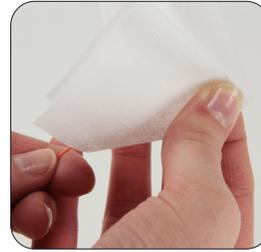
4: Clean the fiber with a lint-free wipe and fiber preparation fluid.
