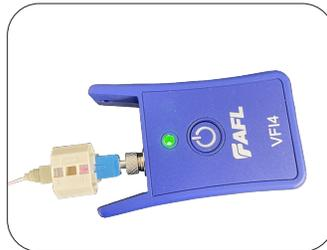
6b: Insert the fiber into the connector. Bring 250  $\mu$ m protective tubing forward. Create a slight bend in the fiber to maintain connection. The light will dim when a connection is made.
