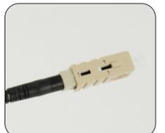
**12:** Screw the boot on completely. Termination is complete.
