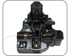
**6:** Set the fiber on the cleaver at the 10.5 mm recommended cleave length (minimum 10 mm). Cleave the fiber.
