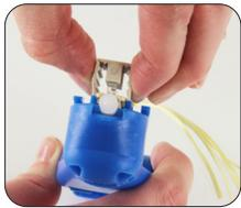
**9:** Disengage the wedge by squeezing both sides while the connector remains in the assembly tool.
