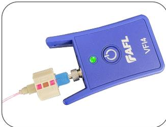
5b: Remove the dust cap. Insert the connector into the VFI. Window 1 of the wedge clip will glow red.
