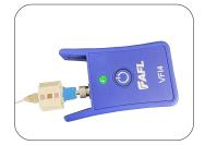
**6b:** Insert the fiber into the connector. Bring 250 μm protective tubing forward. Create a slight bend in the fiber to maintain connection. The light will dim when a connection is made.
