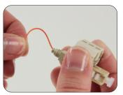
2: Insert the fiber into the connector with the mark facing up. (Reference the strip template for mark placement specific to connector type, SC/ST or LC). Create a slight bend in the connector to maintain connection. (If using the optional VFI Method, see step 6b on page 2.)
