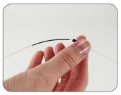
1: Insert the black protective tubing, 250 µm protective tubing and 900 µm boot onto the fiber.
