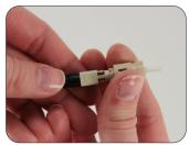
Before applying the connector housing to the connector body, ensure optical connection by the VFI or other suitable method. After the ST housing is applied, you will not be able to release/re-engage the wedge clip if resetting the fiber is required.
