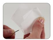
3: Clean the fiber with a lint-free wipe and fiber preparation fluid.
