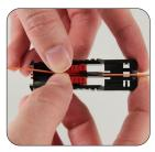
1: If you are using a 900 µm fanout/breakout kit, place into 900 µm cable clamp about 10" from the end of the cable.
