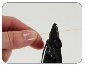
2: Strip 35 mm of 250 µm coating from the fiber. (Refer to template image on bottom of page 3 for length references or use actual cleave length template card for measurements.)
