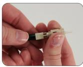
Before applying the connector housing to the connector body, ensure optical connection by the VFI or other suitable method. After the ST housing is applied, you will not be able to release/re-engage the wedge clip if resetting the fiber is required.
