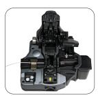
5: Set the fiber on the cleaver at the 10.5 mm recommended cleave length (minimum 10 mm). Cleave the fiber.
