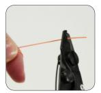
3: Strip 35 mm of 900 µm and 250 µm coating off. (Refer to template image below for length references or use actual cleave length template card for measurements.)
