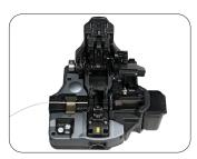
4: Set the fiber on the cleaver at the 10.5 mm recommended cleave length (minimum 10 mm). Cleave the fiber.
