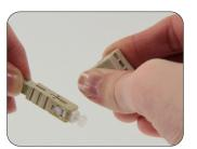
3: Release the wedge clip by squeezing both sides. Remove the wedge clip.
