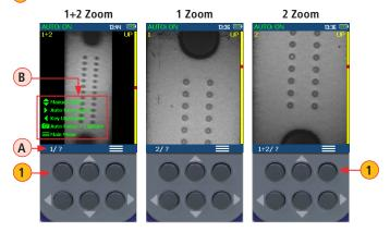
Press to display the Main menu that allows the user to set preferences, manage saved test results and perform other non-test functions.
