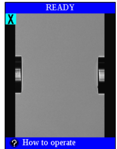
Figure 31 – Best fiber loading position for splicing before tapering.
