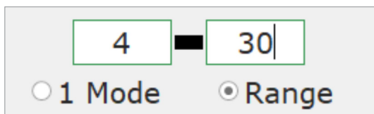
Figure 53 – Example of using the range mode to receive modes 4-30 from the splicer
