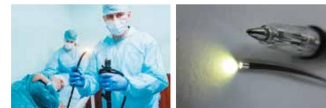
Example: CMOS endoscopy camera with extremely narrow diameter of φ1.3mm
