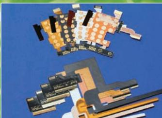
Our flexible printed circuit boards use a polyimide-based CCL and coverlays and are used in single, double, triple, and quadruple layer boards
