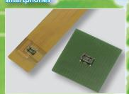
Low profile board-to-FPC stacking connector with compact stacking height of 0.7mm and 0.35 mm pitch connections Helps save board space.
