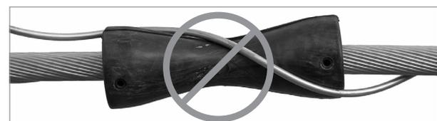
FIGURE 4: Incorrect—Do not wrap around insert
