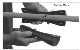
FIGURE 2: Center insert on mark
