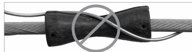
**FIGURE 4: Incorrect—Do not wrap around insert**
