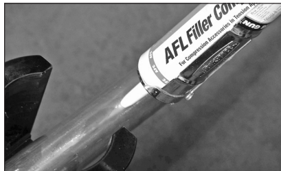
FIGURE 9: Inject AFCHT Filler Compound into the filler hole.
