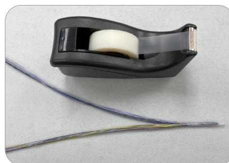
Figure 4b – Taped fiber ends
