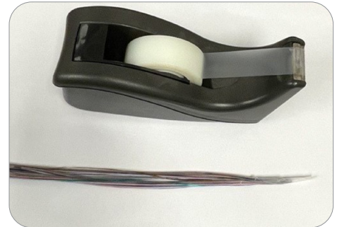
Figure 3c – Taping fiber ends
