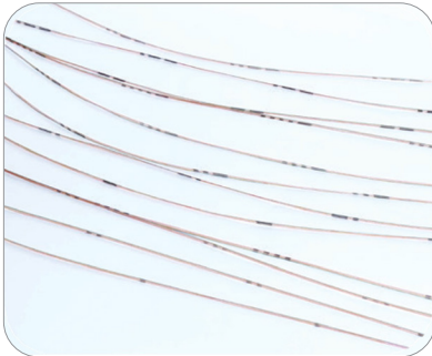
Figure 3a – Fibers with band markings
