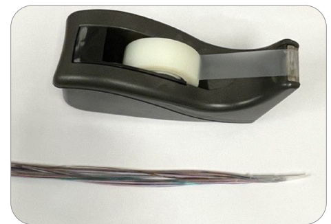
Figure 2b – Taped fiber ends
