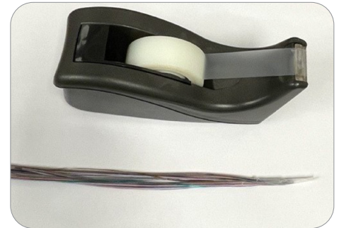
Figure 5c – Taping fiber ends
