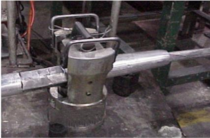
Make initial compression on either side of Joint starting at the "Start" knurl. Make the second compression on the opposite end of the joint at the other "Start" knurl. Continue making compressions to the end of the joint. **Overlap each successive compression by approximately 0.50 inch (1.27 cm). Do not "skip bite." Complete die closure is required for each compression.** Go back and complete the compressions on the opposite end. The center portion of the Joint is not compressed.
