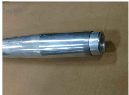
**NOTE:** If the splice body uses filler sleeves, mark the conductor past half of the splice body at a distance equal to the filler sleeve protrusion.
