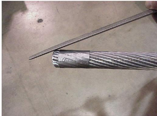
Straighten several feet of the conductor removing the set caused by the reel.
