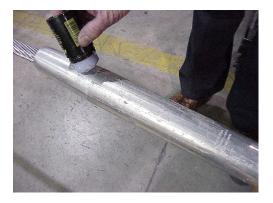
Lubricate area to be compressed from "Start" knurl to end of barrel as illustrated. Lubricate both ends of Joint.
