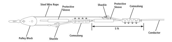
LOAD RATING:Maximum tension limit is 50% of the rated strength of the OPGW or 5,000 pounds,<br/>whichever value is smaller.WARNING:Comealongs are not intended for use as dead ends and are not recommended to hold<br/>conductors at sag tension limits for longer than 6 hours.
