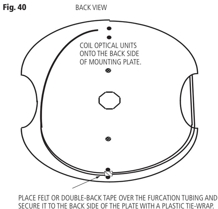
**17.2** Proceed to coil the small section of furcated fibers in a counter-clockwise direction. Align and position the units within the enclosure.
