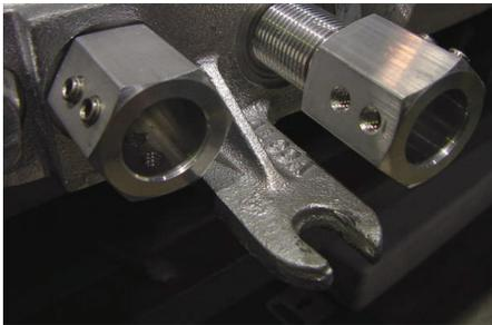
1. Remove the cable retainers (wire retainer) from each connector body.
