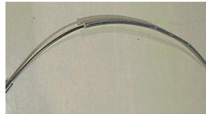
**8.6** Place a mark on the stainless steel tube that represents the removal location.
