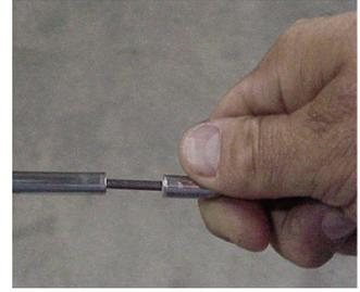
**8.5** All remaining aluminum pipe sections except for a 2" portion shall be ring cut and slid to the end/or removed from the stainless steel tube in 6 to 10 inch sections (see Figs. 17 and 18). Always maintain control of the sample to prevent kinking of the stainless steel tube.
