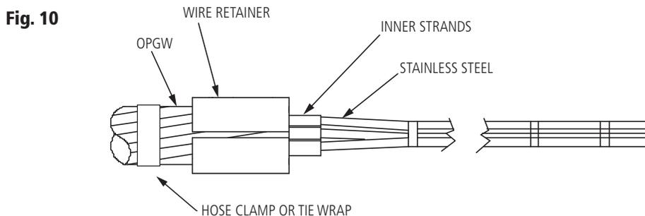
**Note:** The hose clamp or tie wrap can be removed after the wire retainer has been applied
