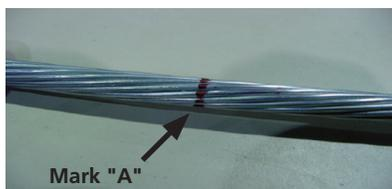
**Note:** Mark "A" is the actual measured length of the cable to the bottom of the connector body as if the enclosure were mounted at the final structure location.
