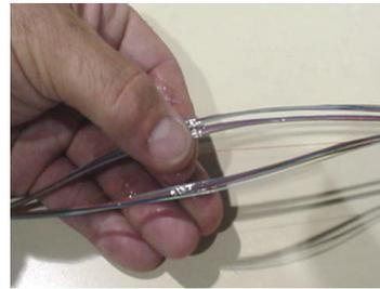
**11.3** Locate one of the colored string binders then lightly pull it until the bundle starts to separate from the other fibers (see Fig. 25 and 26).
