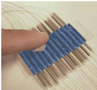
6.1 AFL recommends using the Fujikura 60 mm (#500065) splice sleeves for this application.
