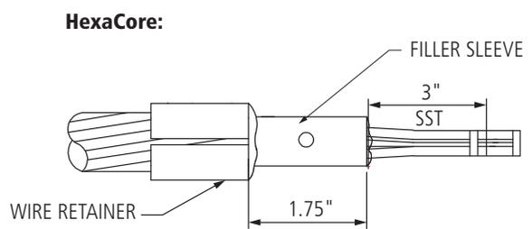
**9.5** Using a heat gun, evenly shrink the tubing around the stainless steel tube and fibers. The heat shrink tube will not shrink onto the fibers. Special care should be taken to ensure that the hot air blast does not remain on the optical fibers for an extended period. Allow the tubing to cool for approximately 5 minutes.
