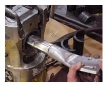
Press the Terminal Connector over the conductor. Make the initial compression at the start knurl. Continue making compressions to the end of the Terminal Connector barrel, overlapping the previous compression by approximately 0.50 inches. Complete die closure is required for each compression.
