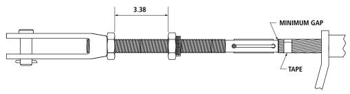
Insert end of conductor into "core grip" of clevis assembly. Rotate clevis assembly "back and forth" while pushing it onto conductor core.
