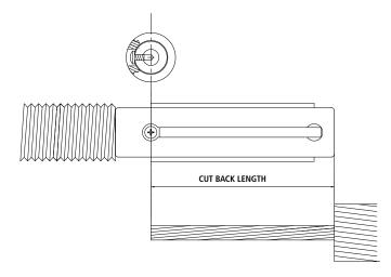
**NOTE:** It is extremely important not to nick the core strands during cutting back of the aluminum strands. If this is done, the ultimate strength of the dead end will be reduced. The cable manufacturer suggests the following method of cutting back the strands.
