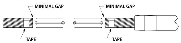
Insert ends of conductor into "Core Grip" ends of steel sleeve. Rotate sleeve "back and forth" while pushing sleeve onto conductor core.
