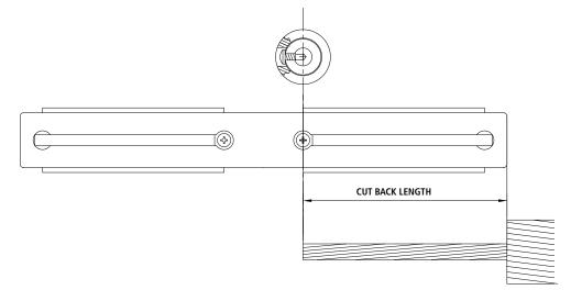
**NOTE:** It is extremely important not to nick the core strands during cutting back of the aluminum strands. If this is done, the ultimate strength of the Joint will be reduced. The cable manufacturer suggests the following method of cutting back the strands.
