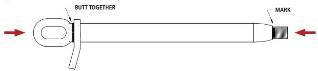
Align eye or clevis in desired orientation of dead end to ensure proper positioning when dead end is fastened to insulator hardware.
