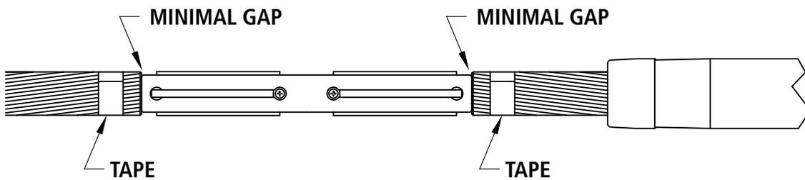
Insert ends of conductor into "Core Grip" ends of steel sleeve. Rotate sleeve "back and forth" while pushing sleeve onto conductor core.
