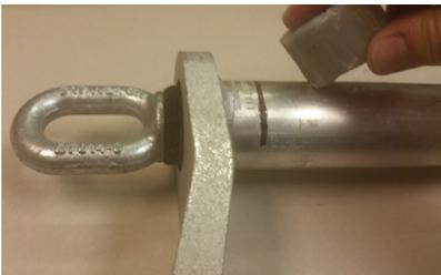
Verify mark place at end of barrel has remained where originally place. If not, push internals together prior to making first compression (see illustration above).
