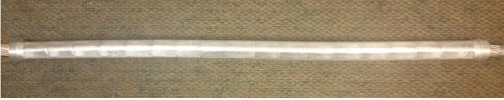
Compressed portion of the joint should have a smooth uniform appearance. Remove flash, if present with file or emery cloth.
