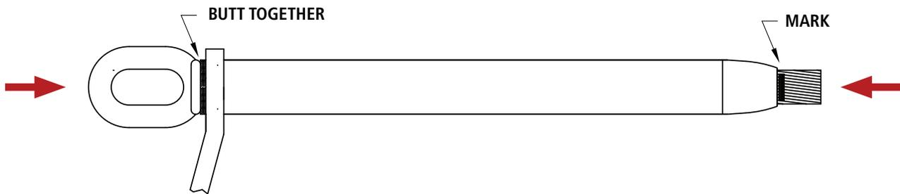
Align eye or clevis in desired orientation of dead end to ensure proper positioning when dead end is fastened to insulator hardware.
