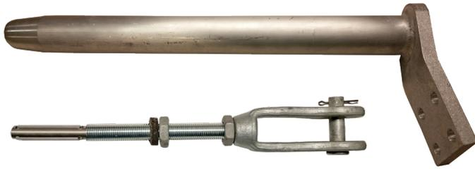
Dead end assemblies consist of an aluminum body and steel adjustable clevis/"core grip". (Felt washer is included as part of clevis assembly.)
