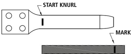
Mark the conductor from the end, a distance equal to the compression length of the terminal.
