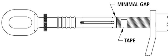
Insert end of conductor into "Core Grip" of Steel Eye. Rotate Eye "back and forth" while pushing Eye onto conductor core.
