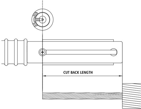
**NOTE:** It is extremely important not to nick the core strands during cutting back of the aluminum strands. If this is done, the ultimate strength of the dead end will be reduced. The cable manufacturer suggests the following method of cutting back the strands.
