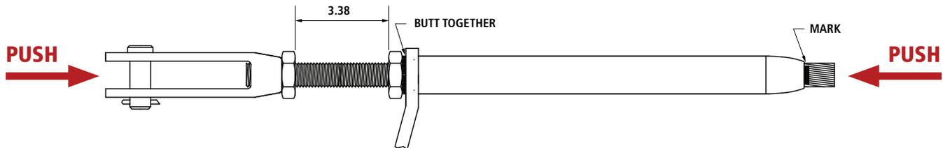
Align clevis in desired orientation of dead end to ensure proper positioning when dead end is fastened to insulator hardware. Lock in place with adjacent jam nut.
