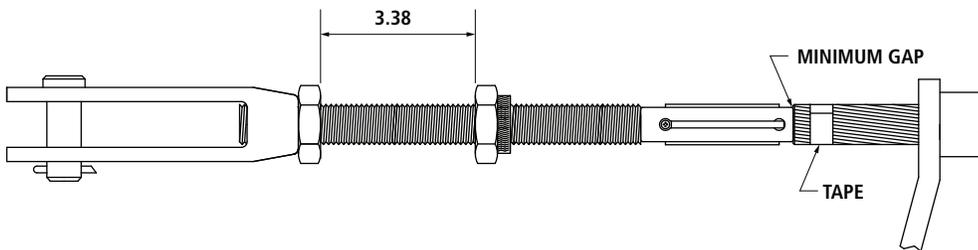
Insert end of conductor into "core grip" of clevis assembly. Rotate clevis assembly "back and forth" while pushing it onto conductor core.
