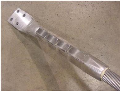
Compressed portion of the Terminal Connector should have a smooth uniform appearance. Remove flash, if present, with file or emery cloth.
