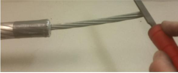
File chamfer on end of core to remove burrs and sharp edge. Chamfer will reduce the expanded diameter of the core (due to cutting) and ease the installation of the Steel Sleeve/"Core Grip".
