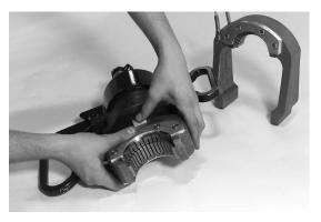
**6.** Remove safety caps from the bottom of power unit and the hose fitting. Insert hose fitting into power unit and tighten to ensure a tight seal.
