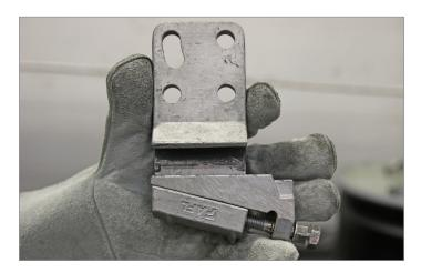
**3.** Place the pad tap connector on the main conductor so that the conductor sits flush in the groove of the wedge.
