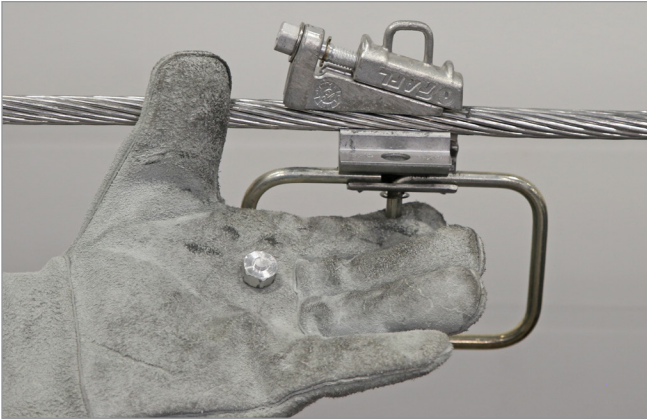
Breakaway bolt head sheared off.
