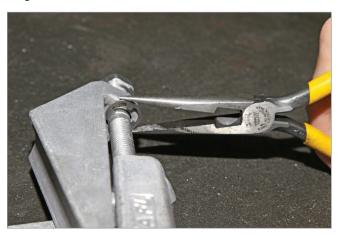
**4.** AFL recommends using a new bolt for reinstallation. See Tables 1 and 2 below. However, if a new bolt is unavailable, the existing bolt can be reinstalled using the corresponding torque values mentioned above.
