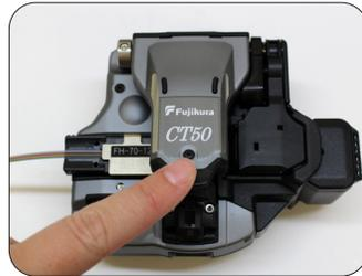
6: Place the fiber holder into the cleaver. The fiber holder should be flush and flat in the cleaver. Cleave the fiber.
