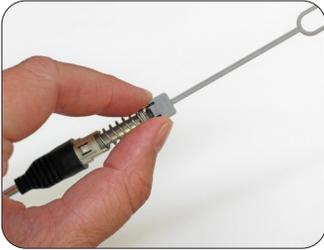
1: Slide the spring unit up to the ferrule and carefully remove the transfer cap by holding onto the ferrule, not the fiber.
