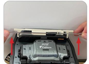
12: Allow the sleeve to cool for ~1 minute. While holding both sides, remove the fiber and sleeve from the heater. Remove the heater attachment by picking up on the edges, avoiding the area that was in contact with the heater.
