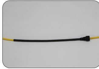
**2:** Insert the boot onto the cordage.
