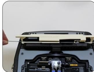
11: While keeping tension on the fiber, turn the assembly 90° and set the heat sleeve, ferrule, and ribbon fiber in the heater attachment with the ferrule going into the square recess on the right and the fiber into the slit on the left. Heat the sleeve.
