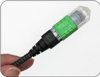
5: Screw the boot unit on completely. Place the dust cap back onto the connector. Installation is complete.
