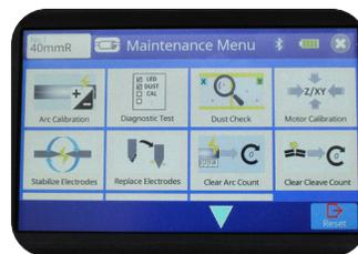
3: Run an arc calibration with the fiber type that you will be splicing to the connector.
