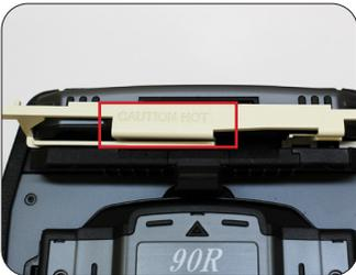
9: Place the provided heater attachment in heater oriented where you can read "CAUTION HOT".
