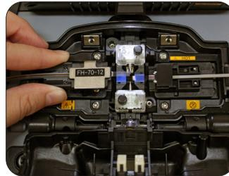
7: Load the fiber holder onto the left side of the splicer and close the cover.
