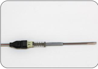
1: Carefully load the ribbon boot spring unit assembly and the heat sleeve onto the ribbon fiber.
