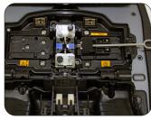
1: Load the ferrule unit holder onto the right side of the splicer. Close the cover.
