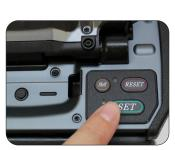
8: Splice the fiber to the FUSEConnect<sup>®</sup> MPO Connector.
