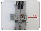
13: When all the fibers are correctly inserted, push the open slider to the left to the closed position. The fibers will push together in a ribbon array.
