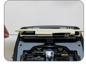
11: While keeping tension on the fiber, turn the assembly 90° and set the heat sleeve, ferrule, and ribbon fiber in the heater attachment with the ferrule going into the square recess on the right and the fiber into the slit on the left. Heat the sleeve.
