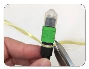
**4**: Trim the excess aramid yarn using the Kevlar scissors.
