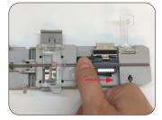
14: Slide your thumb over the fiber to confirm the fiber sits neatly in the fiber holder.
