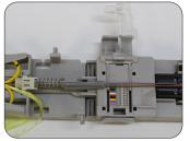
**9:** Carefully insert the spring unit and heat sleeve onto the fibers.
