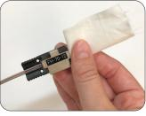
4: Clean the stripped fiber with a lint free cloth and fiber preparation fluid.
