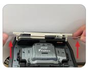
12: Allow the sleeve to cool for ~1 minute. While holding both sides, remove the fiber and sleeve from the heater. Remove the heater attachment by picking up on the edges, avoiding the area that was in contact with the heater.
