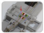
12: Insert the colored fibers through the corresponding color slot with aqua on the left hinge (be careful not to push the lever to the closed position until you have inserted all the fibers correctly).
