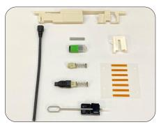
Connector Kit: Heater attachment, cordage tube and boot, ribbon boot and spring unit assembly, spring unit, heat sleeve, housing assembly, ferrule unit, holder, ribbonizing tape and ribbonizing tape jig
