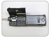
**2**: Place the fiber holder on the hot jacket stripper.
