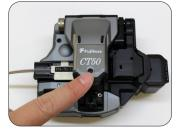
6: Place the fiber holder into the cleaver. The fiber holder should be flush and flat in the cleaver. Cleave the fiber.
