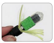
3: Divide the aramid yarn on both sides of the spring unit. Screw the boot  $\frac{3}{4}$  of the way onto the spring unit.
