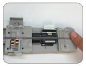
15: While holding the edge of the fiber with your finger, close the clear cover above the fiber holder and confirm that there is no overlapping on the fiber holder.
