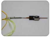
19: Remove the fiber and fiber holder from the ribbonizing tool.
