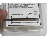
2: Mark the ribbon at 35 mm using the template on the packaging.
