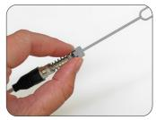
1: Slide the boot and the spring unit up to the ferrule and carefully remove the transfer cap by holding onto the ferrule, not the fiber.
