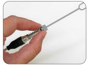
1: Slide the spring unit up to the ferrule and carefully remove the transfer cap by holding onto the ferrule, not the fiber.
