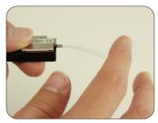
5: Make sure the fibers are dry and separated. Flick the end of the fibers to ensure their integrity.
