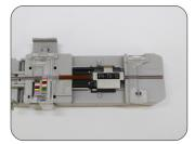
**17**: Carefully attach the ribbonizing tape to the fiber between the fiber holder and the fiber aligner and press lightly.
