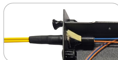
Figure 12. Cap installed over aramid, securing cord
