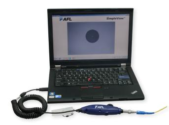
AFL SimpleView Fiber Inspection Software is an application that permits the NOYES DFS1 Digital FiberScope to be used with Windows<sup>®</sup> XP or Windows<sup>®</sup> 7 computers. AFL SimpleView software provides a live, high-resolution video image of the endface of an optical fiber. This capability enables fiber installers and network technicians to inspect and troubleshoot optical fibers and verify that they are clean and undamaged.
