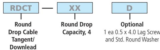
**Ordering Example:** To hold four (4) round drop cables with lag screw hardware kit included, order part number RDCT-4D.
