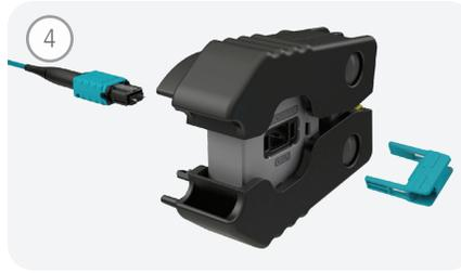
Pull out Pin Exchanger and verify insertion of the pins onto the MTP® PRO connector.
