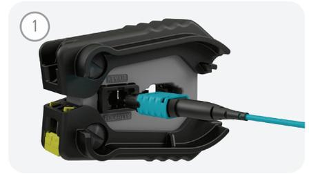
Align key on the MTP® PRO Connector with "KEY UP" on the Polarity Change Port.
