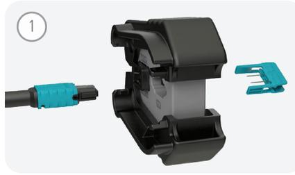
Insert unpinned MTP® PRO Connector in the Pin Change Port until audible "CLICK". **Do not compress the black handles during pin insertion.**
