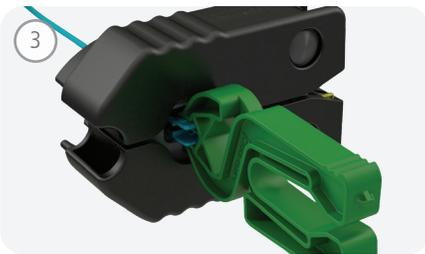
Slide Gripper onto the Pin Exchanger so that it is bottomed and centered. Compress the black MTP® PRO Field Tool handles.
