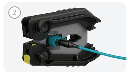
Insert the MTP® PRO Connector in the Polarity Change Port until audible "CLICK".
