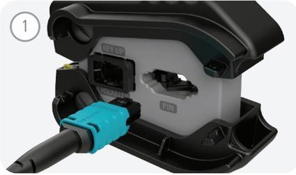
Insert pinned MTP® PRO Connector in the Pin Change Port until audible "CLICK". Do not compress the black handles.
