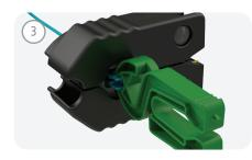
Slide Gripper onto the Pin Exchanger so that it is bottomed and centered. Compress the black MTP® PRO Field Tool handles.
