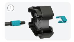
Insert unpinned MTP® PRO Connector in the Pin Change Port until audible "CLICK". Do not compress the black handles during pin insertion.
