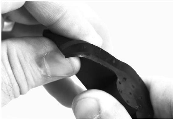
**Photo 6b - Tearing out the Grommet Layers**
