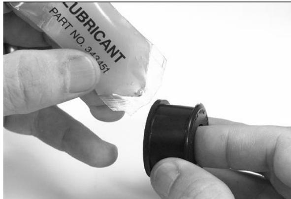
**Photo 8 - Grommet Lubrication**
