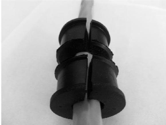
**Photo 9 - Proper Grommet Orientation.**
