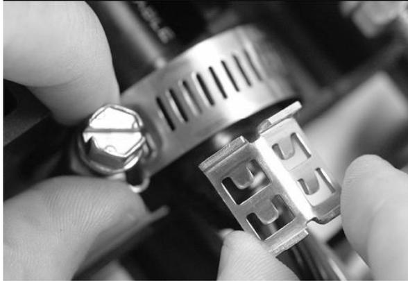
**Photo 14 - Cable Retention Clamp Orientation**
