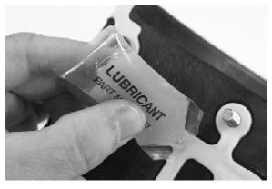
Photo 16 - Lubrication of C-Halves
