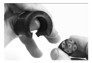
Photo 6c - Grommet with Center Plug and Layers Removed
