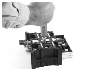
Photo 2 - Cable Clamp Removal from from Center Section
