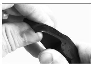
Photo 6b - Tearing out the Grommet Layers
