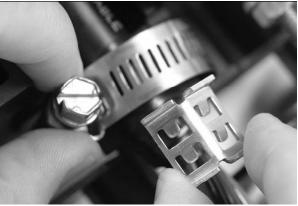
Photo 14 - Cable Retention Clamp Orientation
