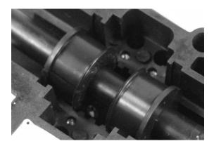
Photo 11 - Cable Sealing Grommet in Center Section
