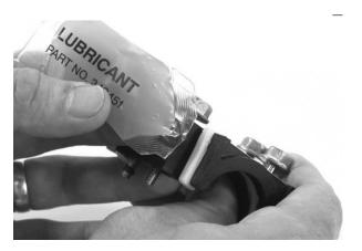
Photo 12 - Lubrication of Cable Clamp
