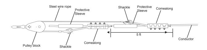
WARNING: Comealongs are not intended for use as dead ends and are not recommended to hold conductors at sag tension limits for longer than 6 hours.
