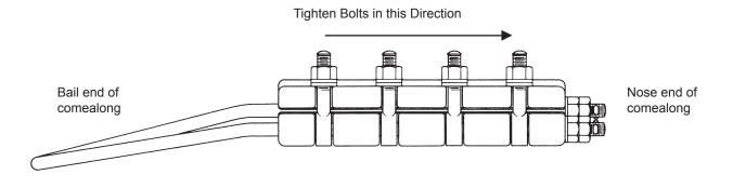
WARNING: Comealongs are not intended for use as dead ends and are not recommended to hold conductors at sag tension limits for longer than 6 hours.
