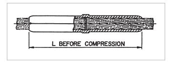
The Quick Compress Jumper Connector is designed for fast and easy installation. By using a high strength alloy, the compression length has been shortened for less compression bites. The jumper connector is pre-filled, eliminating an installation step. Each jumper connector has a center stop, making it easy to center the jumper on the conductor.
