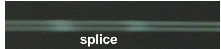
1.5 mm fiber spliced by arc discharge
