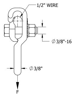
**MATERIAL:** BODY & CLAMP - ALUMINUM BRONZE ASTM B30 **BOLT, NUT & LOCKWASHER - SILICON BRONZE**
