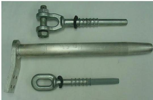
Dead end assemblies consist of an aluminum body and steel eye or clevis forging. (Felt washer is included as part of forging.)
