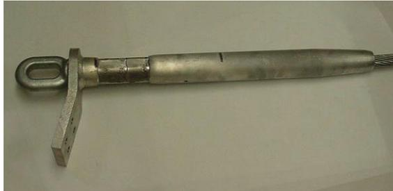
Press the dead end body over the conductor. Lubricate area to be compressed from "Start" knurl to end of barrel. Make the initial compression at the start knurl. Continue making compressions to the end of the dead end body, overlapping the previous compression by approximately .50 inches. Complete die closure is required for each compression.
