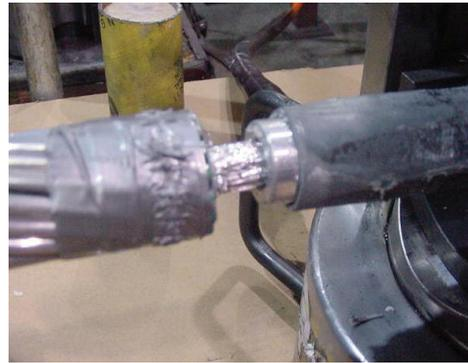
Aluminum sleeve will extrude beyond end of steel barrel. The illustration shown in Fig. 12 is typical after compression.
