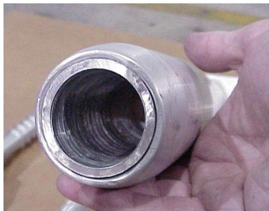
Dead end aluminum bodies may have factory installed (fixed) aluminum sleeves. The sleeves are necessary to provide the proper "Area Reduction" over the conductor.
