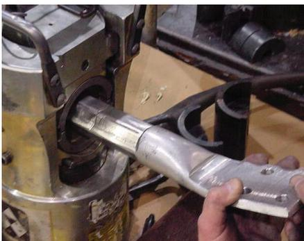
Filler compound should be visible at end of the barrel during the final compressions if adequate amount has been applied. Compressed portion of the terminal connector should have a smooth uniform appearance. Remove flash, if present, with file or emery cloth (see Fig. 20).
