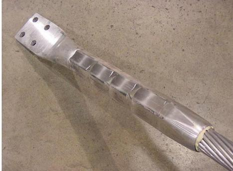
Clean contact surface of terminal connector and dead end pad.
