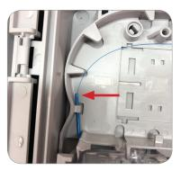
Proper placement of drop buffer tube
