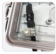
Secure drop cable with clip and grommet
