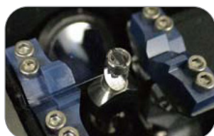
Mirror unit between the fibre ends observes fibre in the axial direction.
